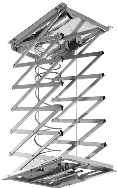
Upper frame to be mounted on ceiling via four oblong slots 12 x 20 mm, with complete electrical appliances, cable guide, concertina elements and lower frame with projector holder.
