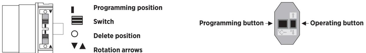
If necessary, the position of the switch on the motor head must be checked or changed. See attached motor manual.
