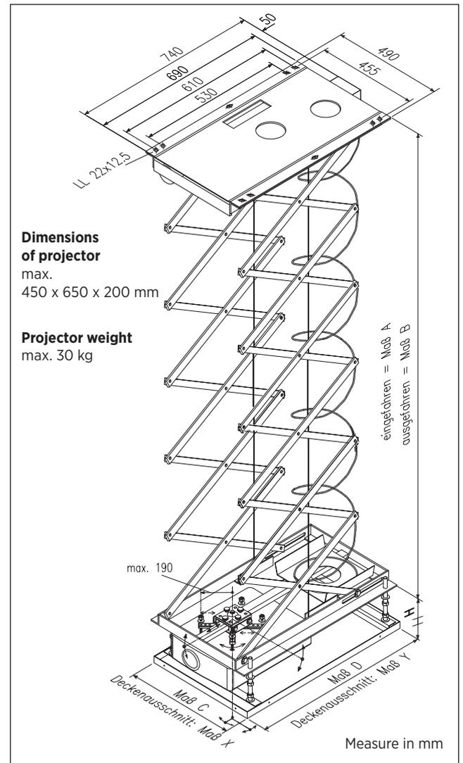
Measure H = projector height + min. 50 mm distance to ceiling plate
