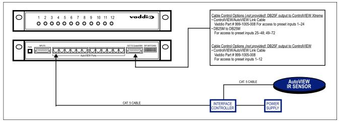
Figure 1 – AutoVIEW Control Expander front and rear panels with connectivity detail.
