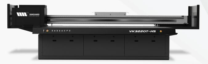
The VK3220T-HS redefines the meaning of productivity on a 3.2 x 2 meter (126" x 80") UV-LED flatbed. With up to three rows of printheads, print speeds can reach over 3,800 square feet per hour. Utilizing 4 picoliter drop size Kyocera heads and a high-speed magnetic drive, there's no compromise on speed to achieve remarkable quality. With the ability to print up to 10cm thick, the only limitation is your imagination.
